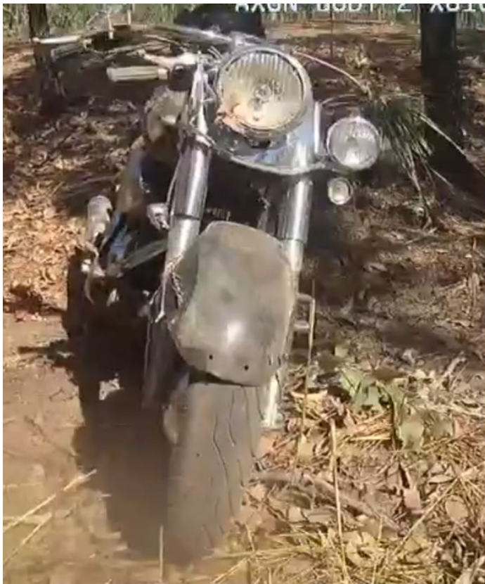
Front forks appeared intact. Front tyre looks like it lacks tread, but this could be due to the bike sliding on the gravel verge of the road when it tipped and skidded.
