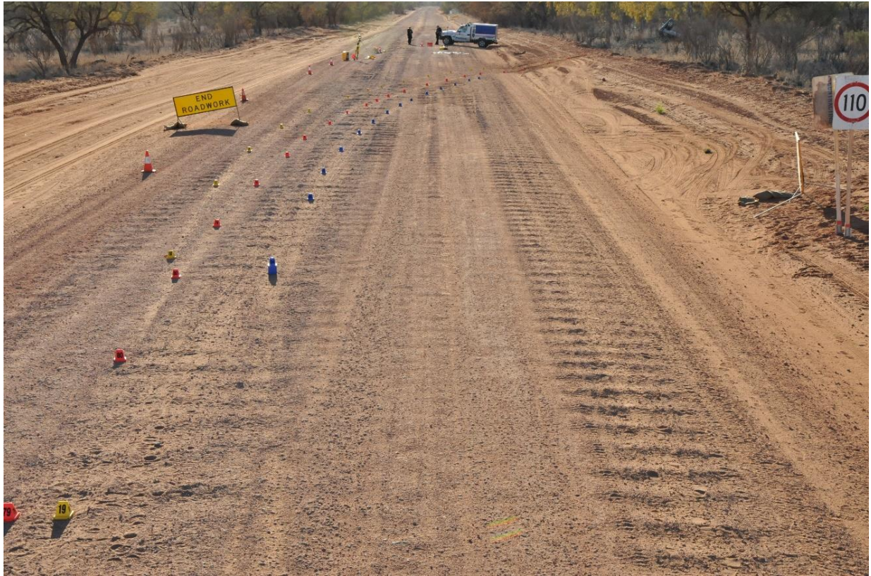
Photo 6: Identification of tyre marks leading to wreckage.
