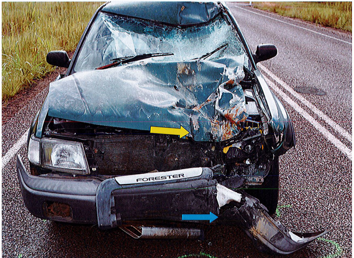
Image 1 - Yellow arrow indicates impression in bonnet from motorcycle front fork. Blue arrow indicates damage caused by motorcycle front wheel
