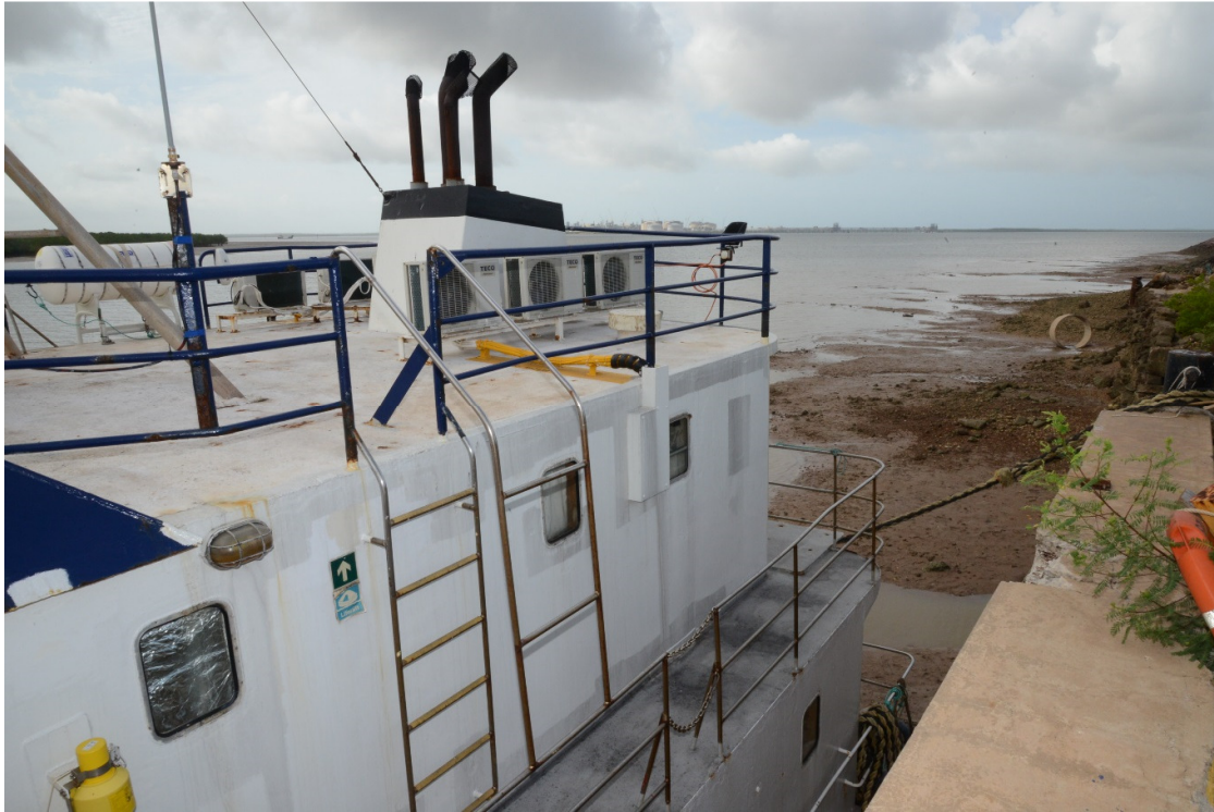
Photo 1 Showing the railing and ladder used for support while stepping from the barge to the wall.
