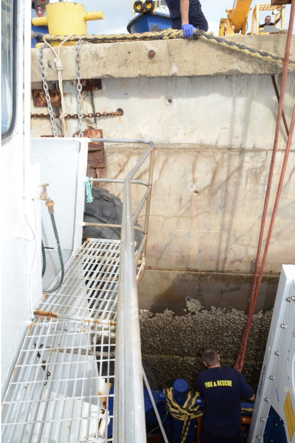
Photo 3 showing the bridge wing, tyre and chains and the distance to the top of the wall
